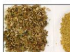
Figure 6 Example of separated stover and kernel fractions using the water separation technique.
